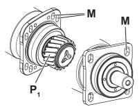
The gearbox can be optionally equipped with an output pinion  $[P_1]$ . The gearing backlash between output pinion and toothed rack / counter-wheel can be adjusted using the slotted holes [M] and the lateral guides. An additional adjustment mechanism is no longer necessary.
