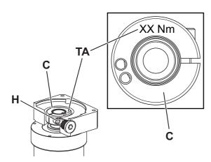
The tightening torque value [TA] of the clamping bolt [H] can be found on the clamping hub [C].
