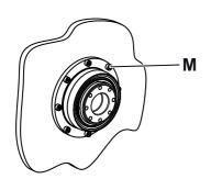
(i) If your gearbox is equipped with reverse centering for motor-side installation [M] on a machine, you will find more information in the separate manual "Reverse centering device for motor-side installation" (doc. no. 2022–D063062). The manual will be provided by our Sales / Customer Service department on request. Please always provide the serial number.
