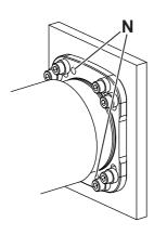
Optionally, there are two bore holes [N] on the gear housing for pinning the gearbox to the machine. You can fasten the gearbox to the machine with cylinder pins.
